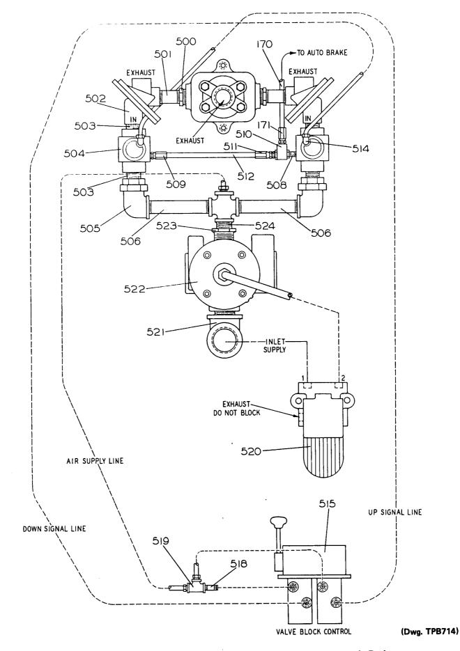
Piping Diagram for 12UWB Winch with Remote Control and Automatic Brake
