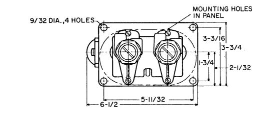
HANDLE NORMALLY ON RIGHT-HAND SIDE DRAWING ROTATED 180° TO SHOW PORT CONFIGURATION
