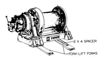
Lifting Method Utilizing A Fork Llft With Forks Beneath Winch Base.
