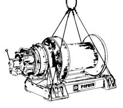
"Four-Point" Lifting Method Utilizing Existing Lifting Eyes
