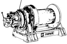
No Attempt Should Be Made to Lift the Winch Using Gear Case Lifting Eye.
