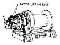
Motor Lifting Eyes Are For Installation And Removal of MOTOR ASSEMBLY ONLY. No Attempt Should Be Made To Lift The Winch Using These Eyes. FGEAR CASE LIFTING EYE
