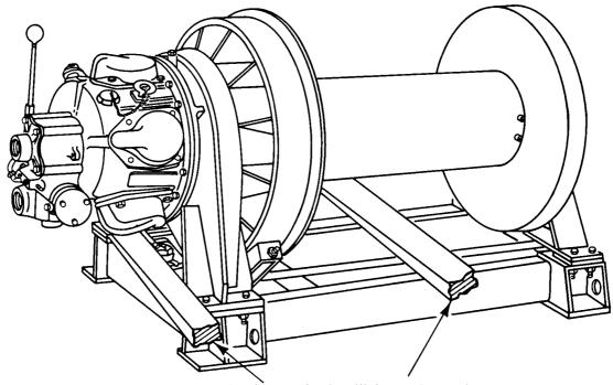
Lifting Method Utilizing A Fork Lift With One Fork Beneath Winch Drum And The Other Beneath The Motor
