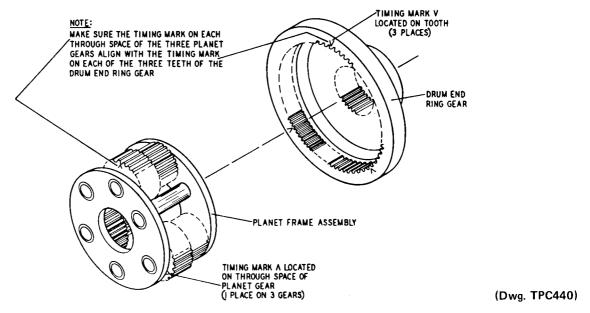
To maintain the proper timing of the gear train when inserting the Planet Gear Frame Assembly (84) into the Drum End Ring Gear (81) of the Winch, proceed as follows:
