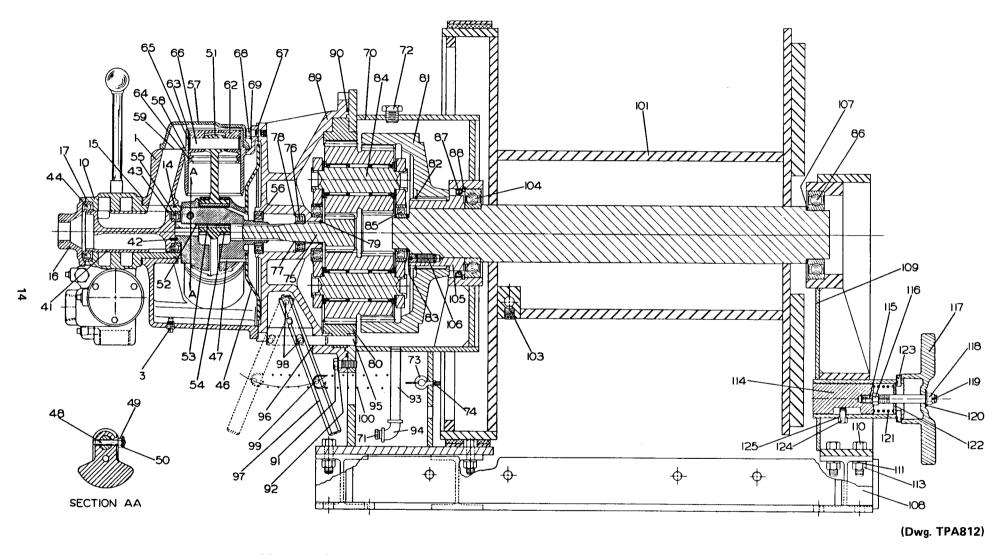
25UWB114 Winch with Manual Throttle, Manual Brake and Disengaging Clutch
