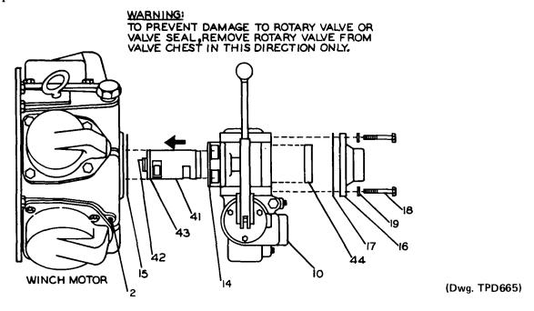
The Rotary Valve (41) incorporates a Seal Ring. The Ring may be replaced separately or with the Rotary Valve. (See illustration above.)
