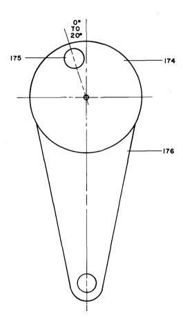
Correct Arrangement of Brake, Crank and Brake Crank Arm
