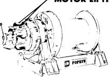
Motor Lifting Eyes Are For Installation And Removal of MOTOR ASSEMBLY ONLY - No Attempt Should Be Made To Lift The Winch Using These Eyes.
