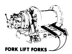
Lifting Method Utilizing A Fork Lift With Forks Beneath Winch Drum.
