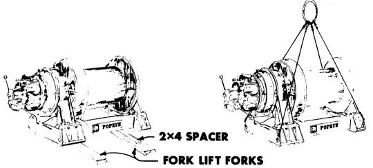
Lifting Method Utilizing A Fork Lift With Forks Beneath Winch Base.
