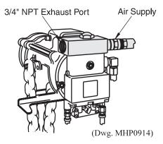
**Quick-Exhaust Valves:** Must be used on all Hoists with Pendant Control when hoses exceed 20 ft (6 m) in length and includes all fittings and clamps. One quick exhaust valve required for each control hose when length exceeds 20 ft (6 m). Two quick exhaust valves required for each control hose when length exceeds 50 ft (15 m).
