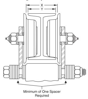
Note: Ensure X - Y = 3/16 to 1/4 inch (5 to 6 mm)
